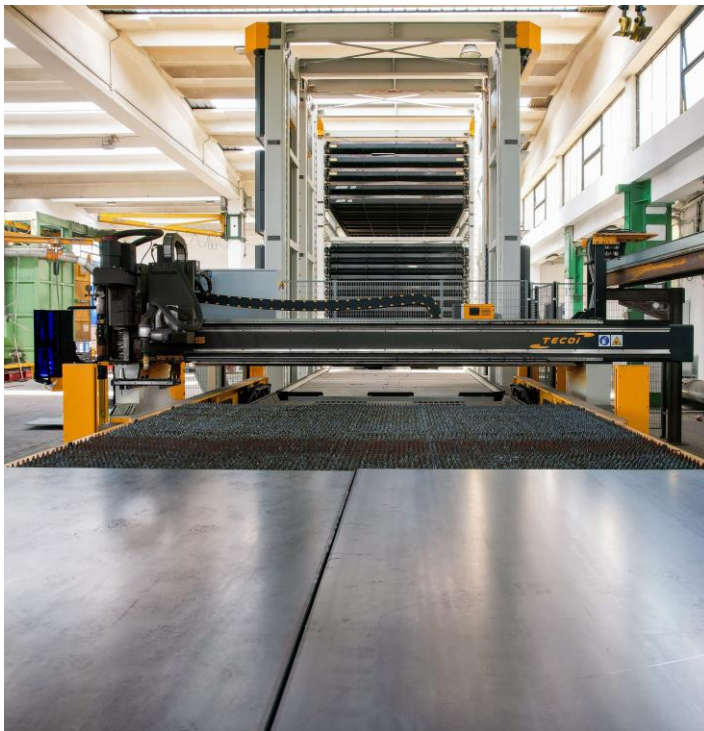
A TECOI TEKNOS with plasma cutting and bevelling as well as drilling capabilities completes ILMEA's new cutting line.
