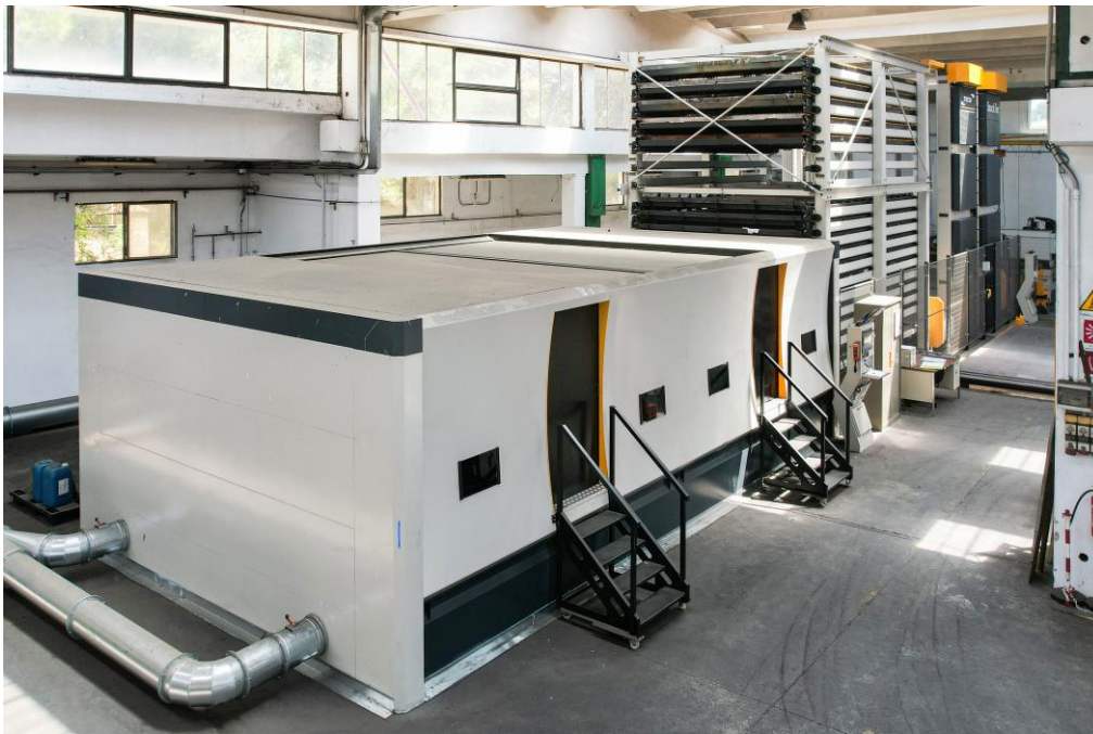
View of ILMEA's LS-CF, equipped with the dual-fibre DFP system developed by TECOI and connected to STOCKTEC.
