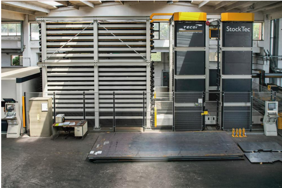
STOCKTEC, the innovative automatic sheet metal storage system that dominates the new ILMEA installation.
